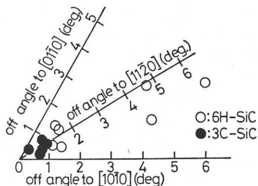
Fig.2, The relationship between polytypes of the grown layers and the magnitude and the direction of off orientation.
