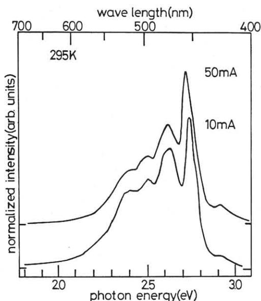
Fig.5, Electroluminescence spectra of a fabricated p-n junction diode.
