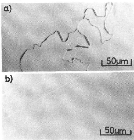
Fig.1, Surface morphology of the grown layers on (a)natural (0001) face (b)off oriented substrates.
