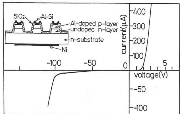
Fig.4, Current-voltage characteristics of a p-n junction diode fabricated using homoepitaxially grown layers of 6H-SiC.
