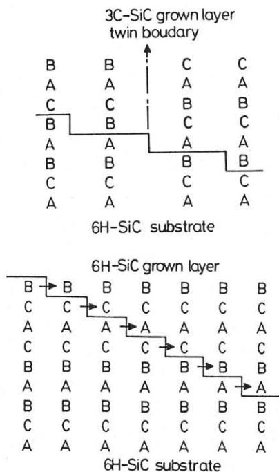
Fig.3, Model of (a)growth of twin crystalline 3C-SiC on well oriented 6H-SiC(0001) (b)homoepitaxial growth on off oriented 6H-SiC(0001).
